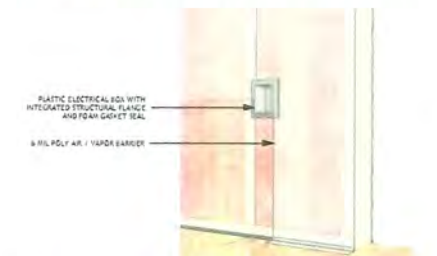
ELECTRICAL BOX INTERFACE
